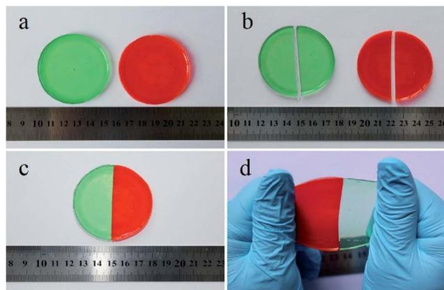
Fig. 1 Self-repairing of PDMS-PUa imaged by using a digital camera at 25 °C: (a) original sample; (b) damaged sample; (c) rejoined sample; (d) self-repairing sample for 48 h. For clear observation, the samples were dyed in red and green.
