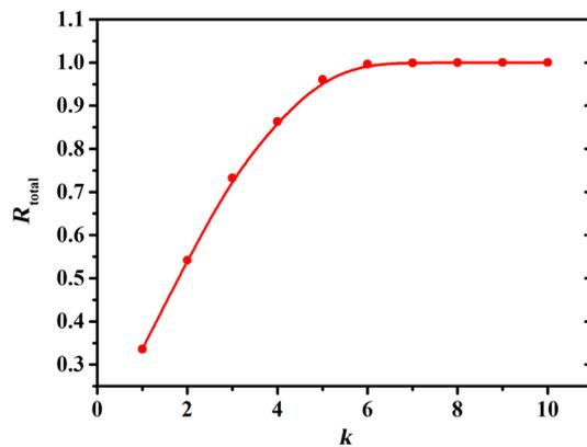
**Fig. 5** Dependence of the optimal NIR (780 to 1100 nm) spectral reflectance ( $R_{\text{total}}$ ) on the number of QWSs ( $k$ ) in the PMMA/PET multilayer heterostructure.
