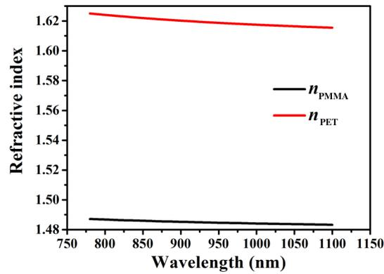
**Fig. 2** Dispersion curves of PMMA and PET in the NIR region.
