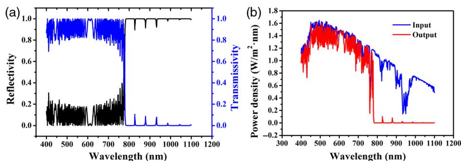
**Fig. 6** (a) The reflectivity and (b) the output spectrum (including incident solar source for comparison) for the designed polymer multilayer heterostructure with six QWSs ( $k = 6$ ).
