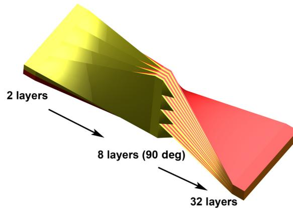
**Fig. 7** The micronano multilayer coextrusion technology based on torsion lamination.
