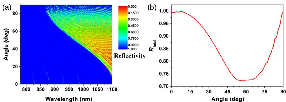
**Fig. 9** (a) The reflectivity  $R_{\text{total}}$  of the designed structure calculated by simulation based on the incident angle and the wavelength and (b) dependence of the reflectance  $R_{\text{total}}$  in the NIR spectrum (780 to 1100 nm) on the incident angle.
