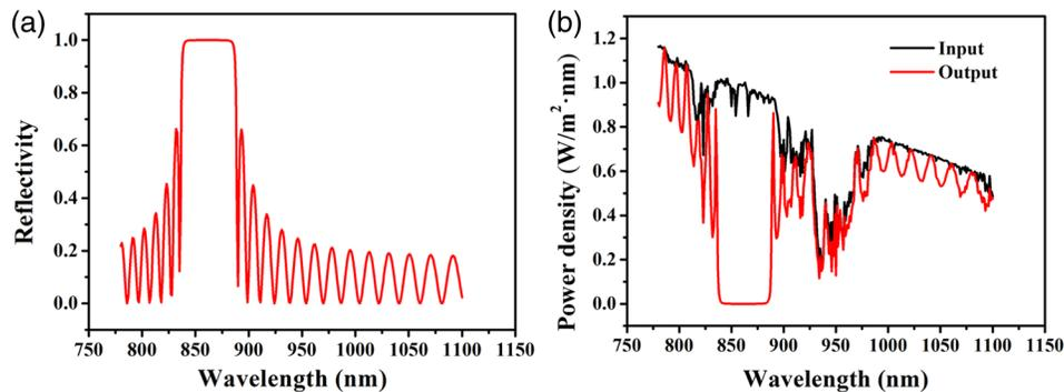
**Fig. 4** (a) The reflectivity and (b) the output spectrum (including incident solar source for comparison) for the designed polymer multilayer heterostructure with only one QWS ( $k = 1$ ).
