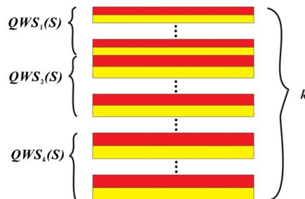
**Fig. 1** Schematic diagram of the multilayer heterostructure consisting of  $k$  PMMA/PET QWSs (each stack contains  $S$  PMMA/PET bilayers).
