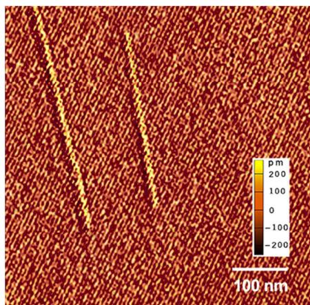
**Figure 2** AFM image (Cypher, Asylum Research, CA) of single PEMA chains adsorbed on the HOPG substrate (scan size: 0.6 μm × 0.6 μm, measured in air). The PEMA chains adopt a train-like conformation on the substrate. The polymer chains are stretched due to the effect of molecular combing in the sample preparation [42]. AFM image of a blank HOPG substrate is shown as a reference in Fig. S3 in the ESM.
