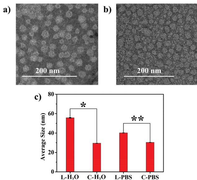
**Fig. 2** TEM images of (a) L micelles and (b) C micelles at a polymer concentration of 0.25 mg ml<sup>-1</sup>. (c) Average size of L and C micelles in H<sub>2</sub>O and PBS (pH 7.4) at a polymer concentration of 0.25 mg ml<sup>-1</sup>. Data are shown as mean  $\pm$  SD ( $n = 3$ ; Student's *t* test, \* $p < 0.01$ , \*\* $p < 0.02$ , both  $p$  values indicate the statistical significance of the diversity between each group).
