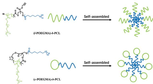
**Scheme 1** Structural formula and schematic illustration of (*l*-POEGMA)-*b*-PCL and (*c*-POEGMA)-*b*-PCL.
