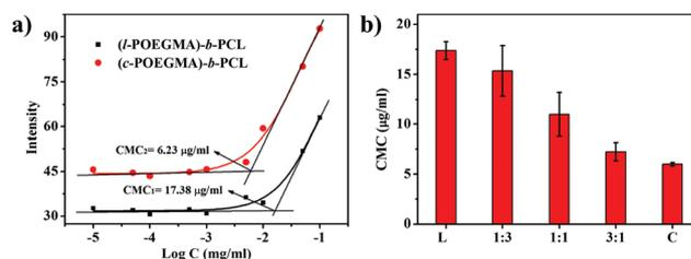
**Fig. 1** (a) The intensity of  $I_{393\text{ nm}}$  in the emission spectra as a function of the logarithm of the concentrations of (*l*-POEGMA)-*b*-PCL and (*c*-POEGMA)-*b*-PCL copolymers, (b) CMC values of L micelles, C micelles and three hybrid micelles. 1 : 3, 1 : 1, and 3 : 1 represent molar ratios (C : L) of 1 : 3, 1 : 1, and 3 : 1 of the (*c*-POEGMA)-*b*-PCL and (*l*-POEGMA)-*b*-PCL copolymers, respectively.
