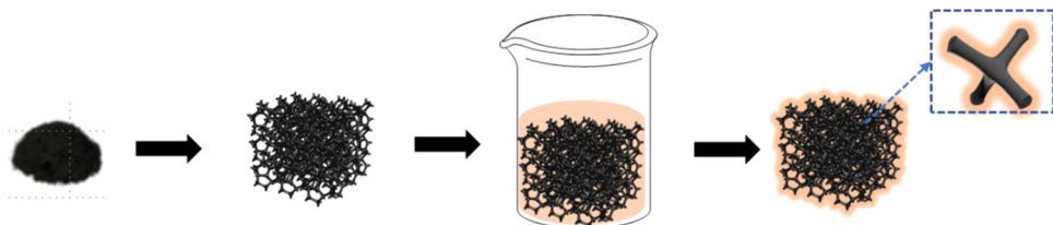
Fig. 10. General preparation process for polymer composites by compounding with a 3D continuous framework.
