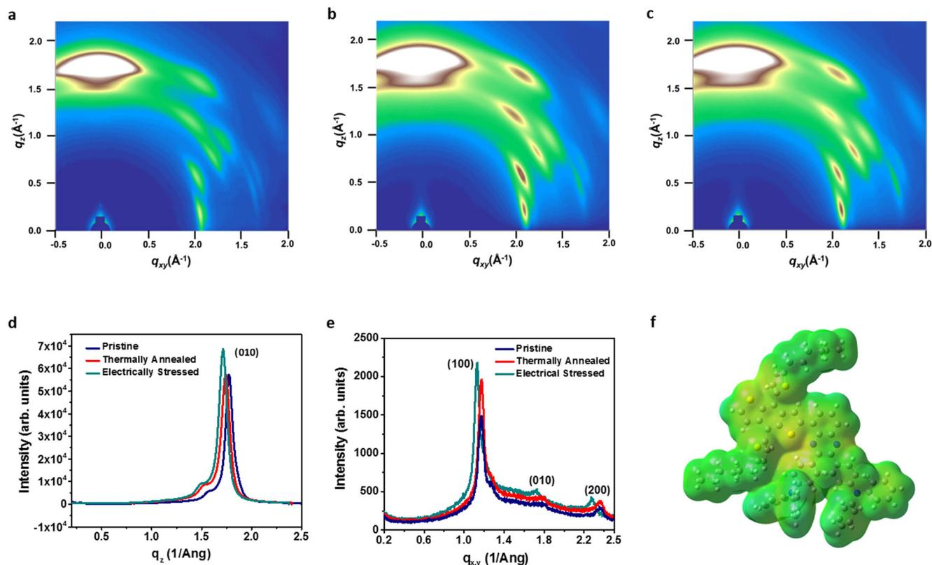
**Fig. 4** Crystallinity of the 2D conjugated polymer. GIWAXS images of the PBDTT-BQTPA thin film **a** in its pristine state, **b** under thermal annealing and **c** upon being subjected to voltage stressing. Line cuts of the GIWAXS of the PBDTT-BQTPA thin film in **d** the out-of-plane direction and **e** the in-plane direction. **f** Electrostatic potential (ESP) surface of the repeating unit of PBDTT-BQTPA derived from molecular simulation.
