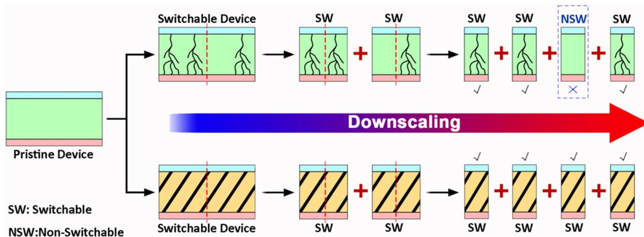
**Fig. 1 Localized and bulk switching mechanisms.** Schematic illustration of the filamentary (upper panel) and bulk phase (lower panel) resistive switching phenomena in polymer memristor devices and their downscaling processes.
