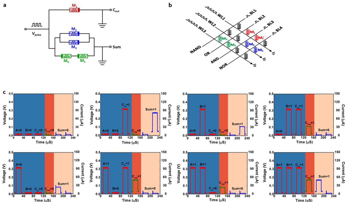
**Fig. 5** Logic operation based on the 2D polymer memristor devices. **a** Circuit design, **b** memristor array representation, and **c** experimental datasets of a parallel 1-bit full adder. The blue area of **c** represents the logic inputs, while the orange and yellow regions represent the bit-carry and sum outputs.
