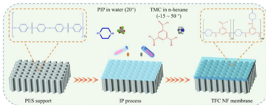
**Figure 1.** Schematic presentation for fabricating TFC NF membranes via the TAIP method.
