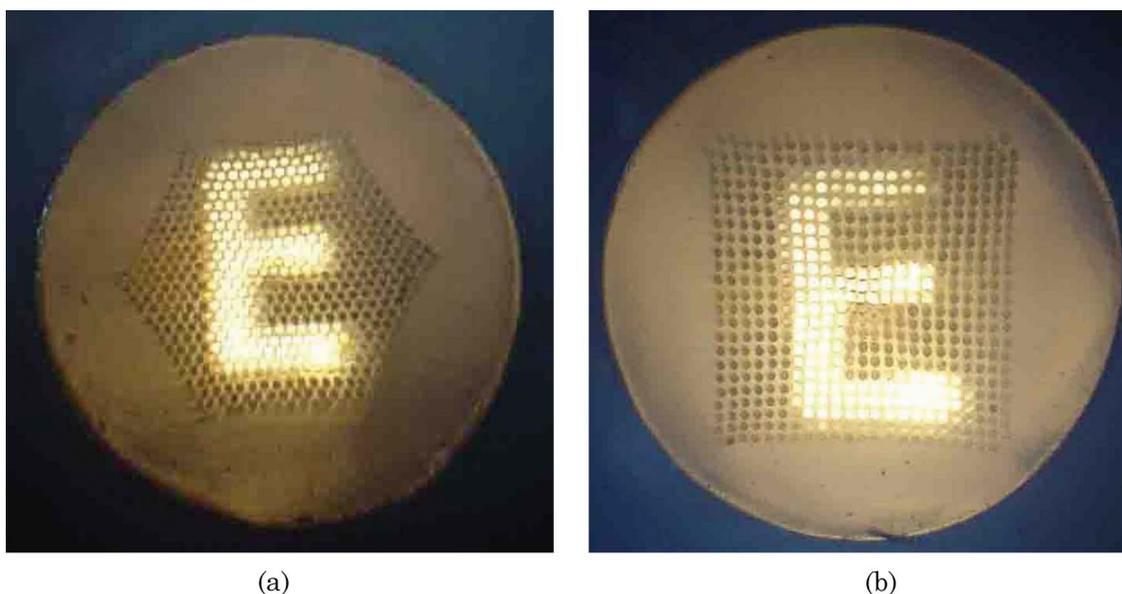
Fig. 5. (Color online) CCD camera images of the "E"-shaped aluminum screen transmitted by (a) a MPOF with a hexagonal array of 547 liquid cores and (b) a MPOF with a rectangular array of 525 liquid cores, respectively.
