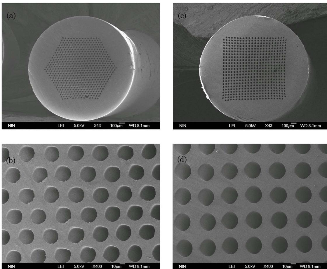
Fig. 1. Scanning electron micrograph of the cleaved end faces of MPOFs. (a) and (b) MPOF with a 547-hole hexagonal array in different magnifications. (c) and (d) MPOF with a 525-hole rectangular array in different magnifications.
