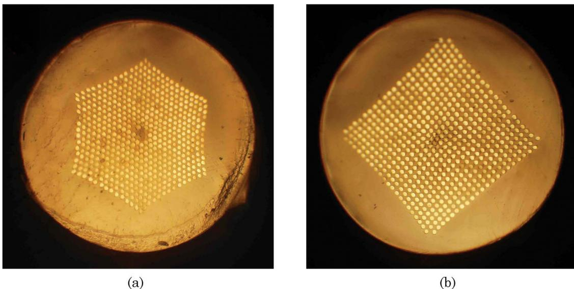
Fig. 3. (Color online) Photos of MLCAFs illuminated on the distal end. (a) Hexagonal array with 547 liquid cores. (b) Rectangular array with 525 liquid cores.
