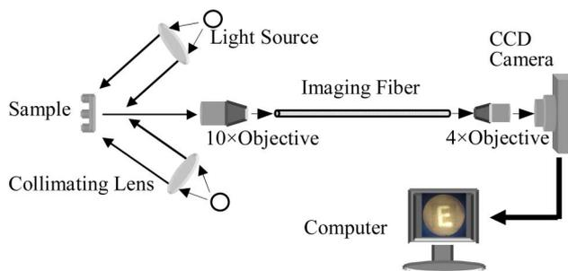
Fig. 4. (Color online) Schematic of the MLCAF imaging system.
