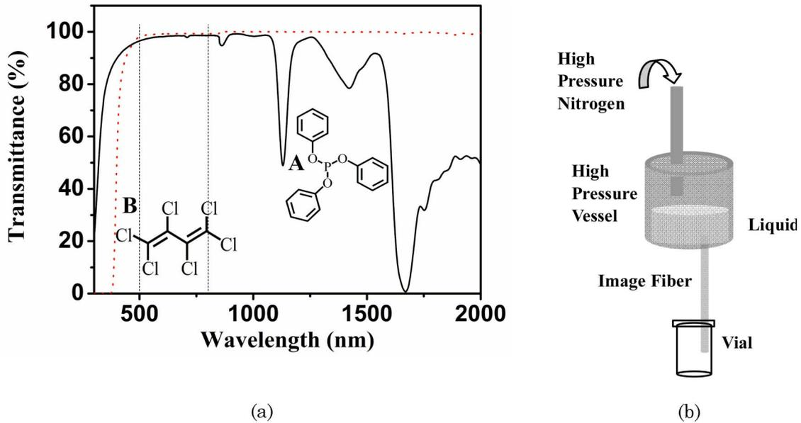
Fig. 2. (Color online) (a) Transmittance of triphenyl phosphite (solid curve) and hexachloro-1, 3-butadiene (dotted curve). (b) Schematic of injecting liquid into the hole array of a fiber.
