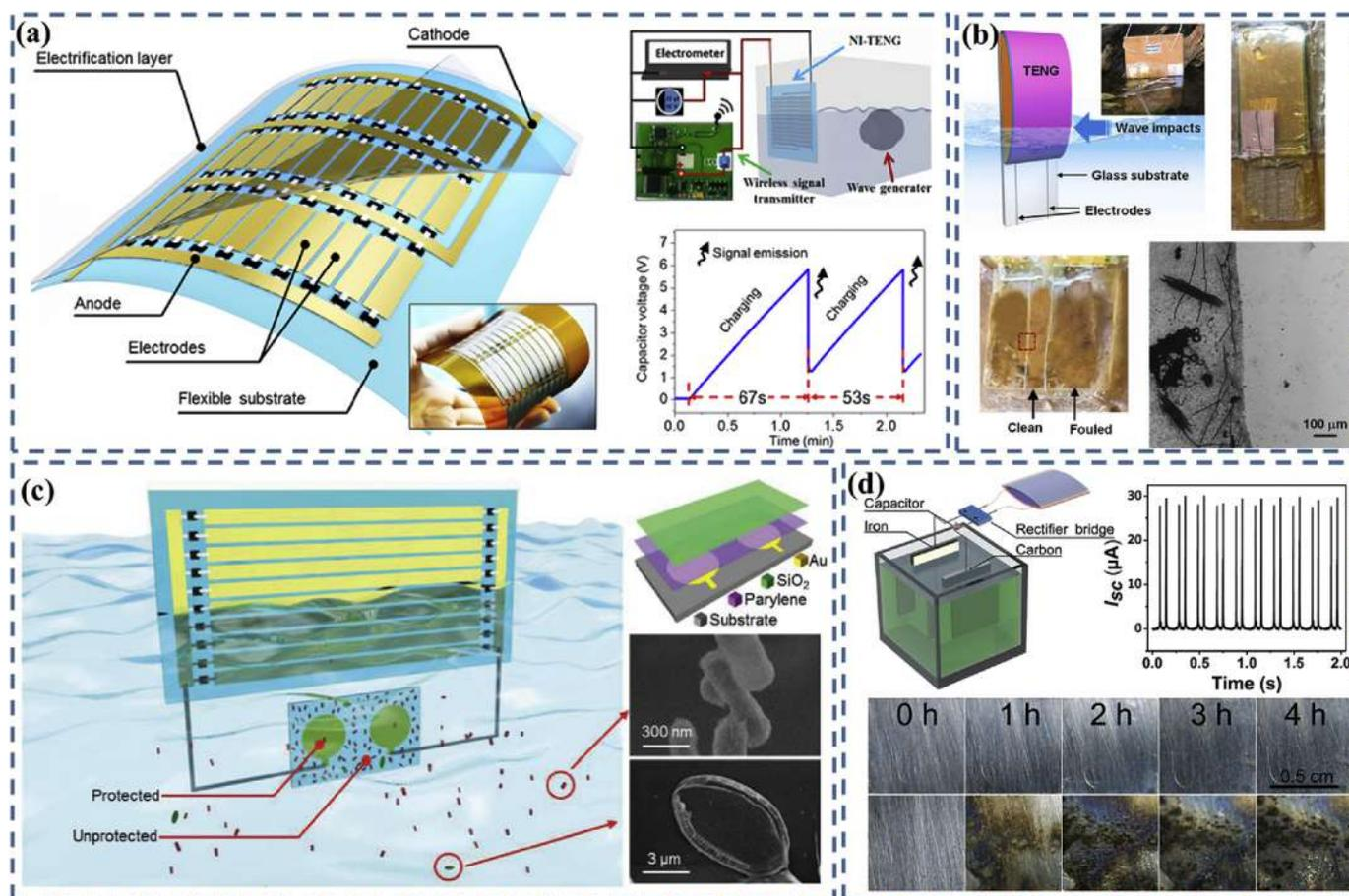
Fig. 5. TENG works on the water for energy harvesting and anti-corrosion. (a) The designed TENG with DC output is used to harvest wave energy for powering a wireless signal transmitter [123].
