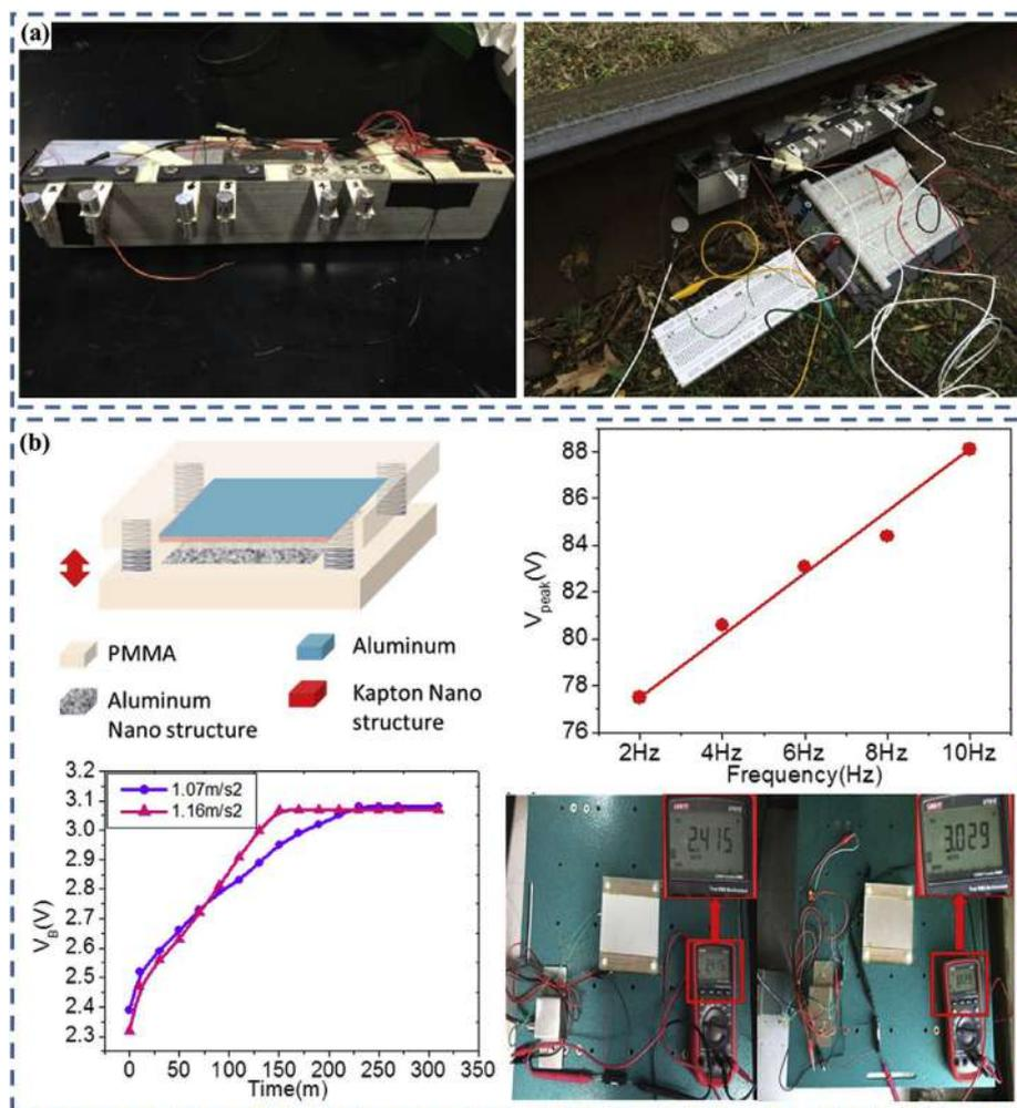
**Fig. 10.** Different methods for vibration energy harvesting of track. (a) Photograph of the device with different cantilever beam length for different frequencies vibration energy harvesting and the experiment test system [180].
