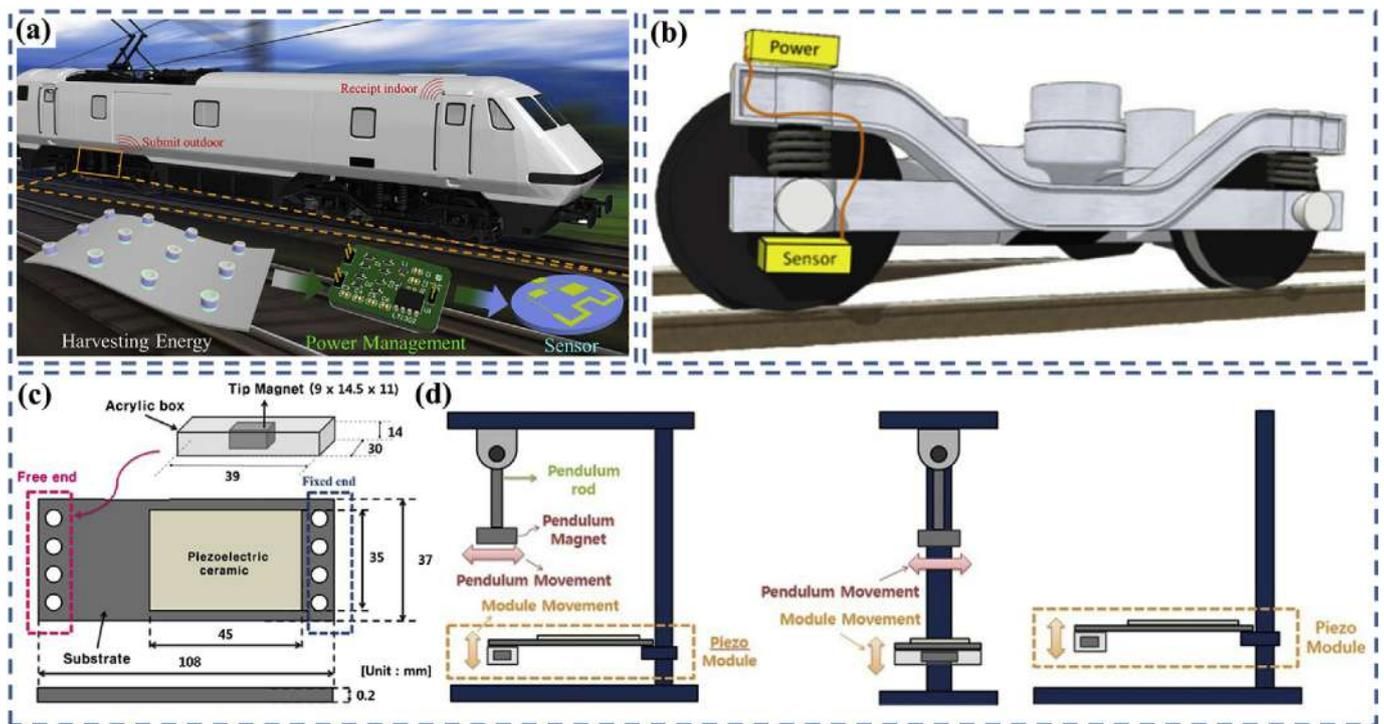
Fig. 3. Energy harvesting technology for train. (a) Self-powered system including TENG, power management and a sensor for train monitoring [116]. (b) Placement of energy harvester on the bogie for a sensor [118]. (c) Design and dimensions of the energy harvesting module. (d) Pendulum moves in the X-direction, Y-direction, vertical vibration [119].
