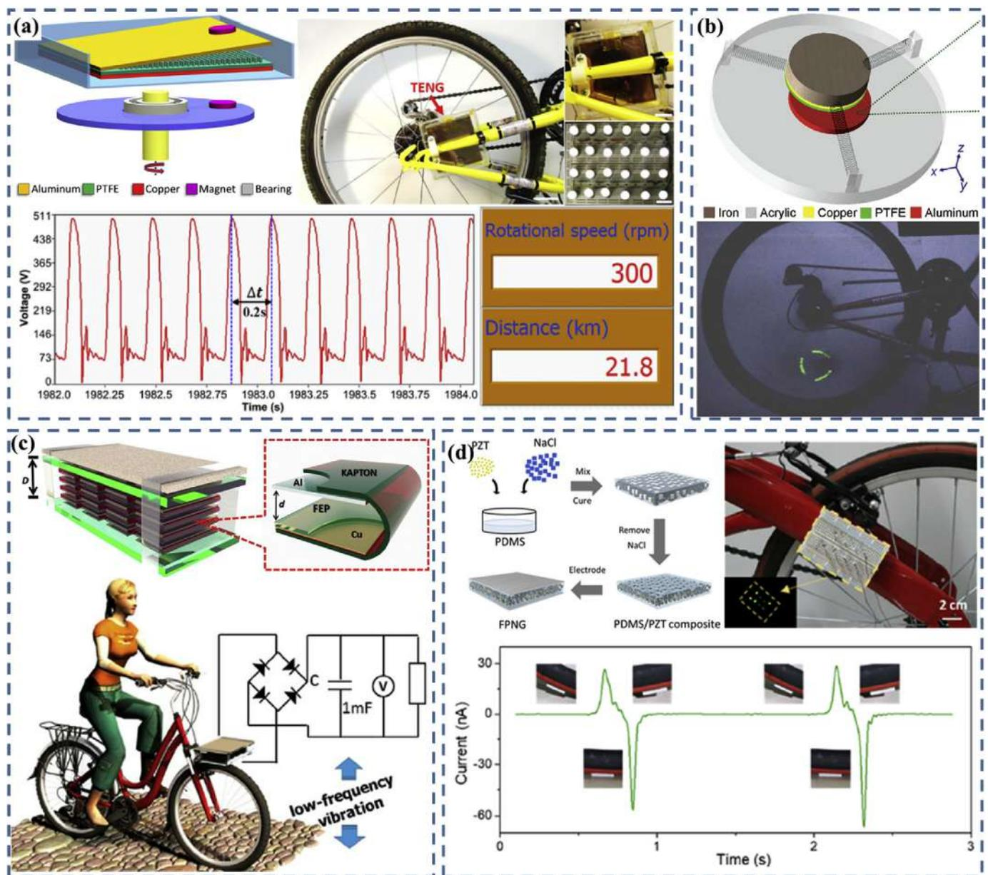
Fig. 4. Nanogenerator applied on bicycle for energy harvesting. (a) Automatic transition TENG applied on bicycle to harvest rotation energy and monitor rotational speed [120].
