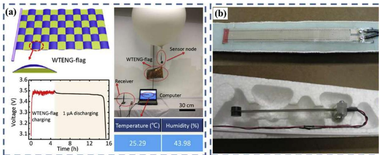
Fig. 6. Energy harvesting application on balloon and unmanned aerial vehicles. (a) The fabricated TENG including nickel and Kapton is used to harvest energy for wireless sensor node [132].
