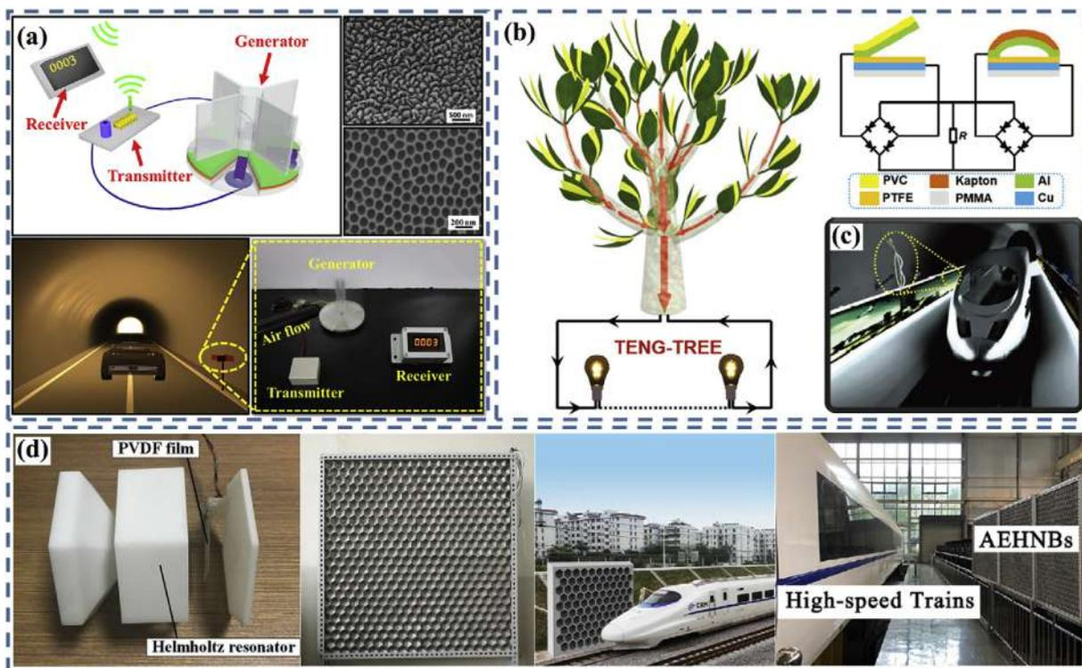
**Fig. 8.** Potential and application on tunnel as a sensor or energy harvester. (a) The wireless traffic volume sensing system by a TENG and an EMG [141]. (b) Diagram of TENG tree with leaf-TENG and stem-TENG. (c) Schematic diagram of TENG tree applied in the tunnel to power the advertising illumination [144]. (d) An energy harvesting unit including the Helmholtz resonator with PVDF film and its application to harvest acoustic energy by running high-speed train [145].
