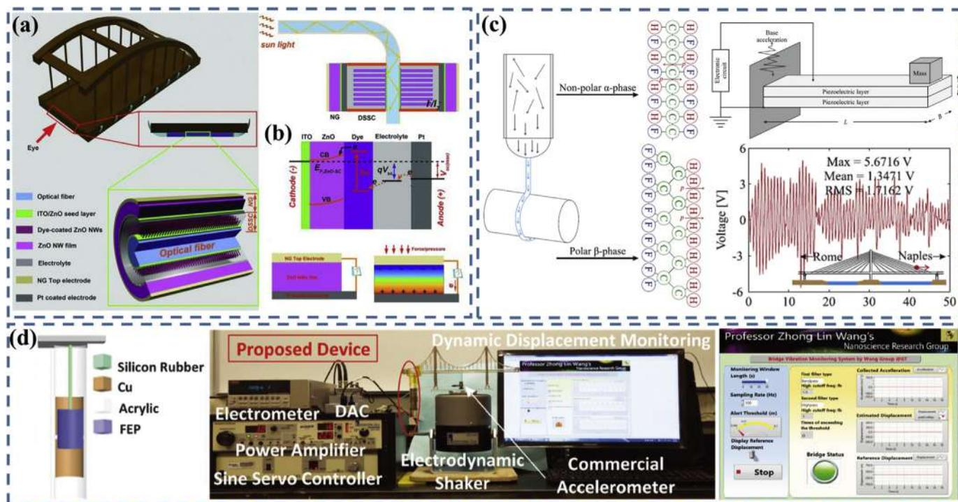
Fig. 7. Self-powered bridge system based on nanogenerator. (a) Bridge as a demonstration for the self-powered nanosystem by hybrid cell, including a solar cell and ZnO NWs based PENG. (b) Working principle diagram of the solar cell and PENG [137]. (c) Bimorph-structure energy harvester by electrospun PVDF nanofibers is used for bridge state monitoring [138]. (d) The typical free-standing mode of TENG as an accelerometer for dynamic bridge vibration monitoring system [140].
